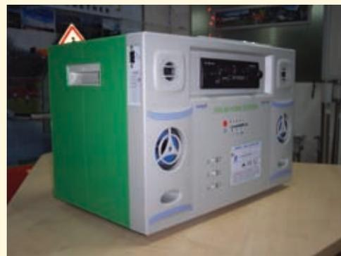
**Beijing Sunpu** developed a new Solar Home System “plug and play” unit built of durable plastic. The plastic casing gives the PV system an attractive appearance and provides room for including a radio, VCD or DVD player, and speakers. Two casing sizes have been developed—one for small systems (10–30 Wp) and one for larger systems (30–60 Wp). The total project cost was Y 572,000 (US\$77,000), with a CG Facility grant of Y 150,000 (US\$20,000).
